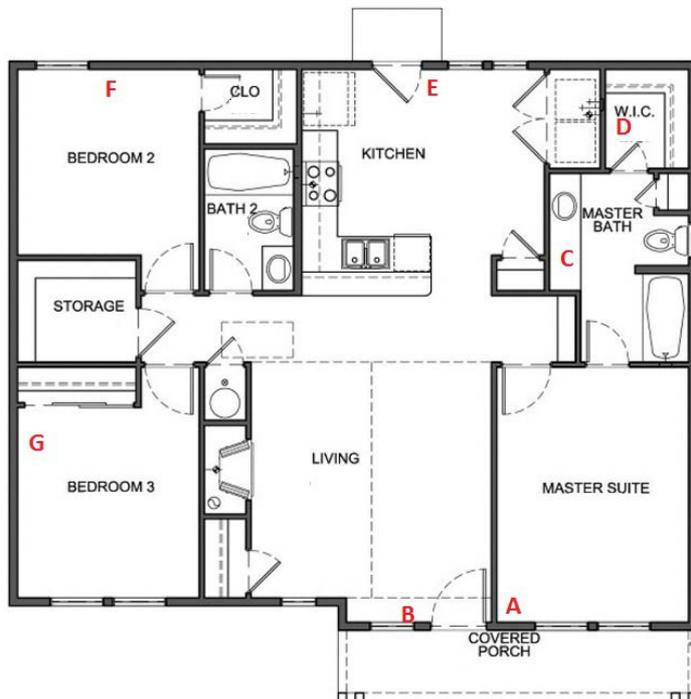
In above illustration A can be both: socket or switch and can control B, C, D, E, F, G even it is not having hard cooper wire connection between them.
