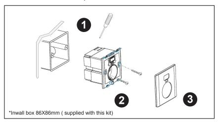
Screw the 6 screws for electrical Wire/cable connection pay attention to connect acording to the signs behind the back cover
