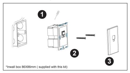
1. Screw the 6 screws for electrical Wire/cable connection pay attention to connect acording to the signs behind the back cover
